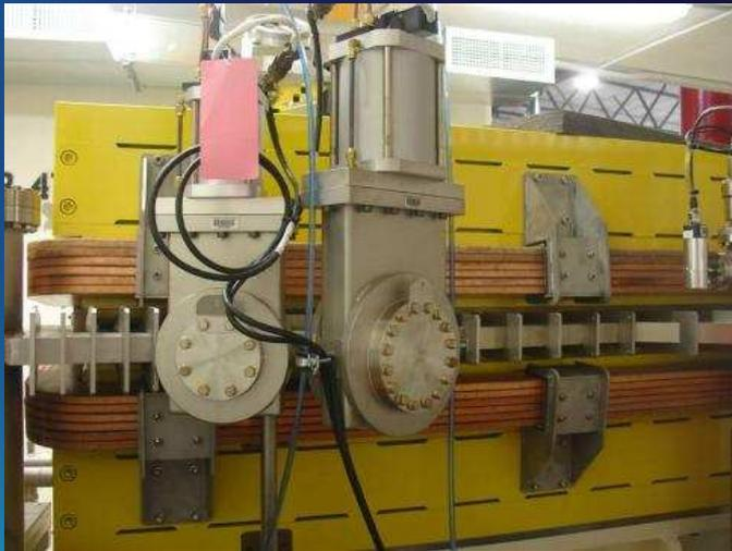
Infrared dipole chamber with vacuum isolation gate valves installed
