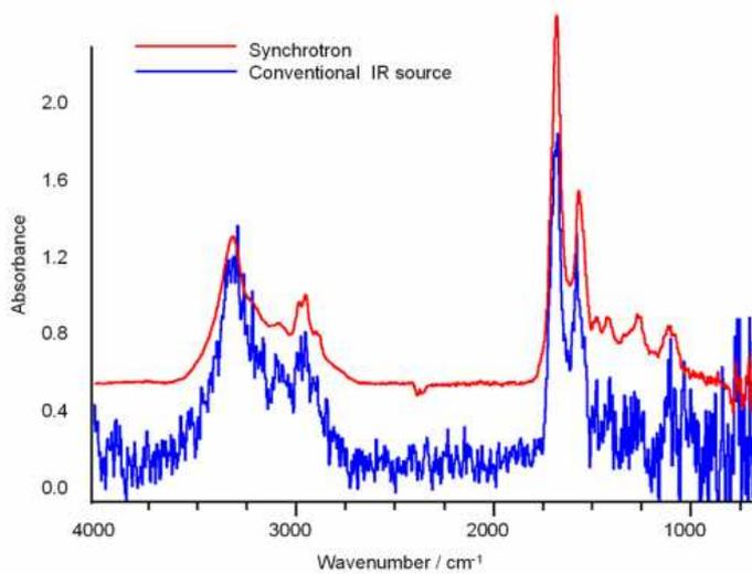
Absorbance spectra of tissue sample recorded at 10 μm spatial resolution under identical collection conditions using a Globar™ infrared source and synchrotron radiation.
