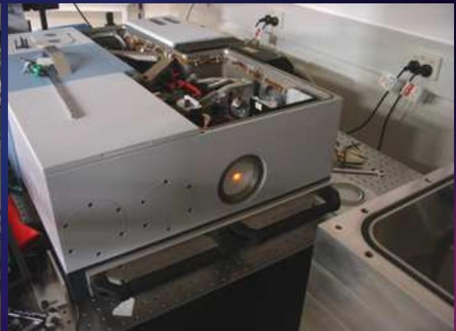
Collimated beam at entrance to FTIR spectrometer
