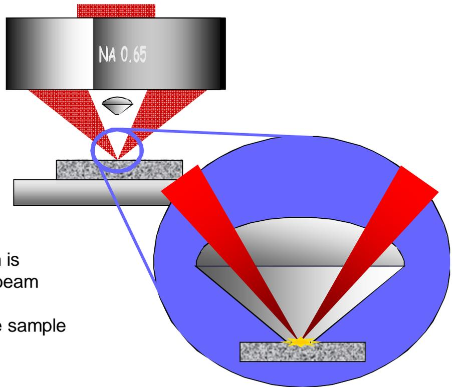
IR absorbance spectrum is generated when the IR beam reflects inside a crystal that is in contact with the sample
