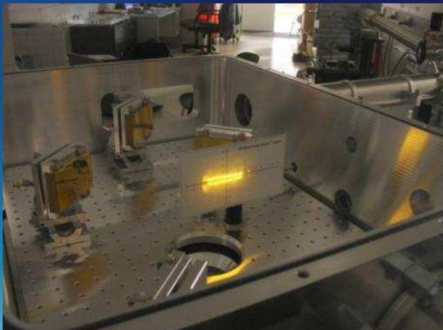
Visible beam profile in Beamsplitter Vessel
