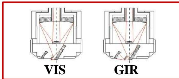
The grazing angle objective provides IR radiation at grazing incidence (65 to 85 degrees) for the analysis of ultra-thin (sub-micron) coatings on metallic substrates.
