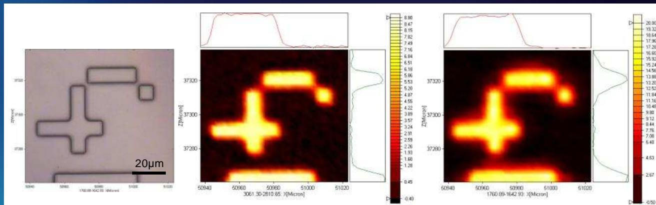
Polymer pattern on  $\text{CaF}_2$  produced by photolithography
