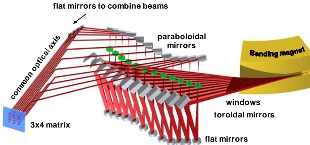
The light from a bending magnet is separated into 12 collimated Synchrotron beams rearranged back into a 3x4 matrix and sent into a IR microscope and spectrometer (48 mirrors in total).
