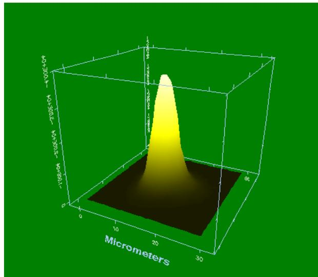
Microscope Beamline at SRS - unapertured beam profile at sample stage. Area mapped = 30x30  $\mu\text{m}$ . Beam halfwidth = 8x8  $\mu\text{m}$ .
