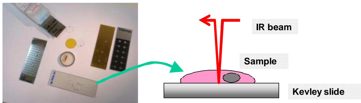
Absorption/reflection (Ag undercoat/SnO<sub>2</sub> overcoat), visible transmission.
