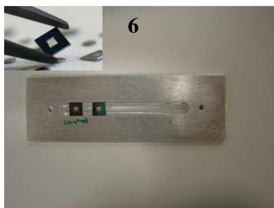
1. Special resolution patterns on mirror slides, for testing the beamline performance.
