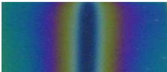
Poly ethylene glycol monolayer gradient on reflective surfaces (eg. ITO glass) can be studied. Understand the mechanism of protein repellent properties of PEG coatings.
