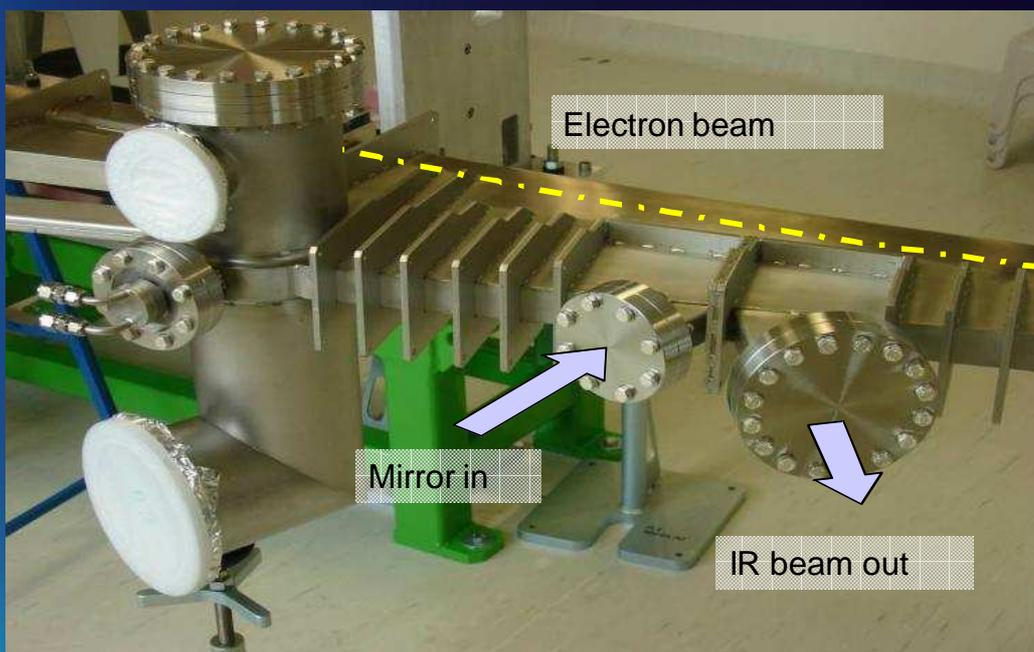
Specially adapted Infrared Dipole Chamber at Australian Synchrotron
