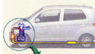
Since its introduction more than 20 years ago, the catalytic converter has sharply reduced automotive emissions. It breaks down harmful carbon monoxide, nitrogen oxides and hydrocarbons
