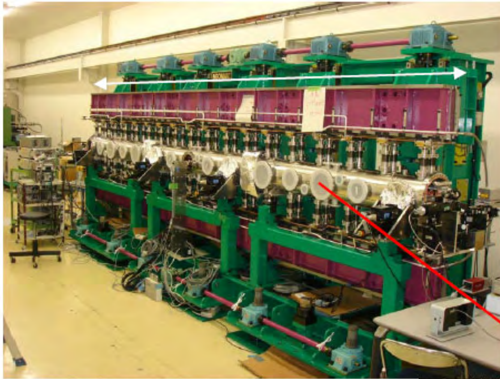
Outlook of 5 m long in-vacuum undulator for X-ray FEL.
