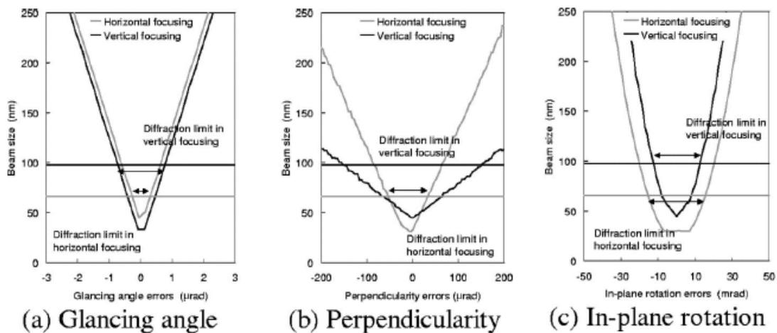
**Figure 4** Tolerance limits of mirror alignments. The vertical axis means geometrical beam size calculated by ray-tracing simulator. The horizontal lines indicate the diffraction limits defined as the distance between the first minima.
