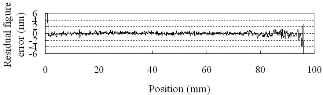
**Figure 3** Typical figure error of an Osaka Mirror. Figure accuracy of 2 nm peak-to-valley can be easily obtained with our fabrication method.
