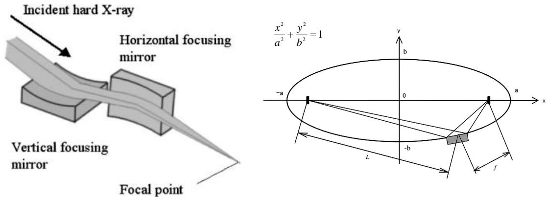
**Figure 1** Kirkpatrick-Baez optics. It consists of two elliptical mirrors aligned perpendicularly to each other. X-rays from a light source placed at one focus are reflected on the mirror surface and always reach the second focus.
