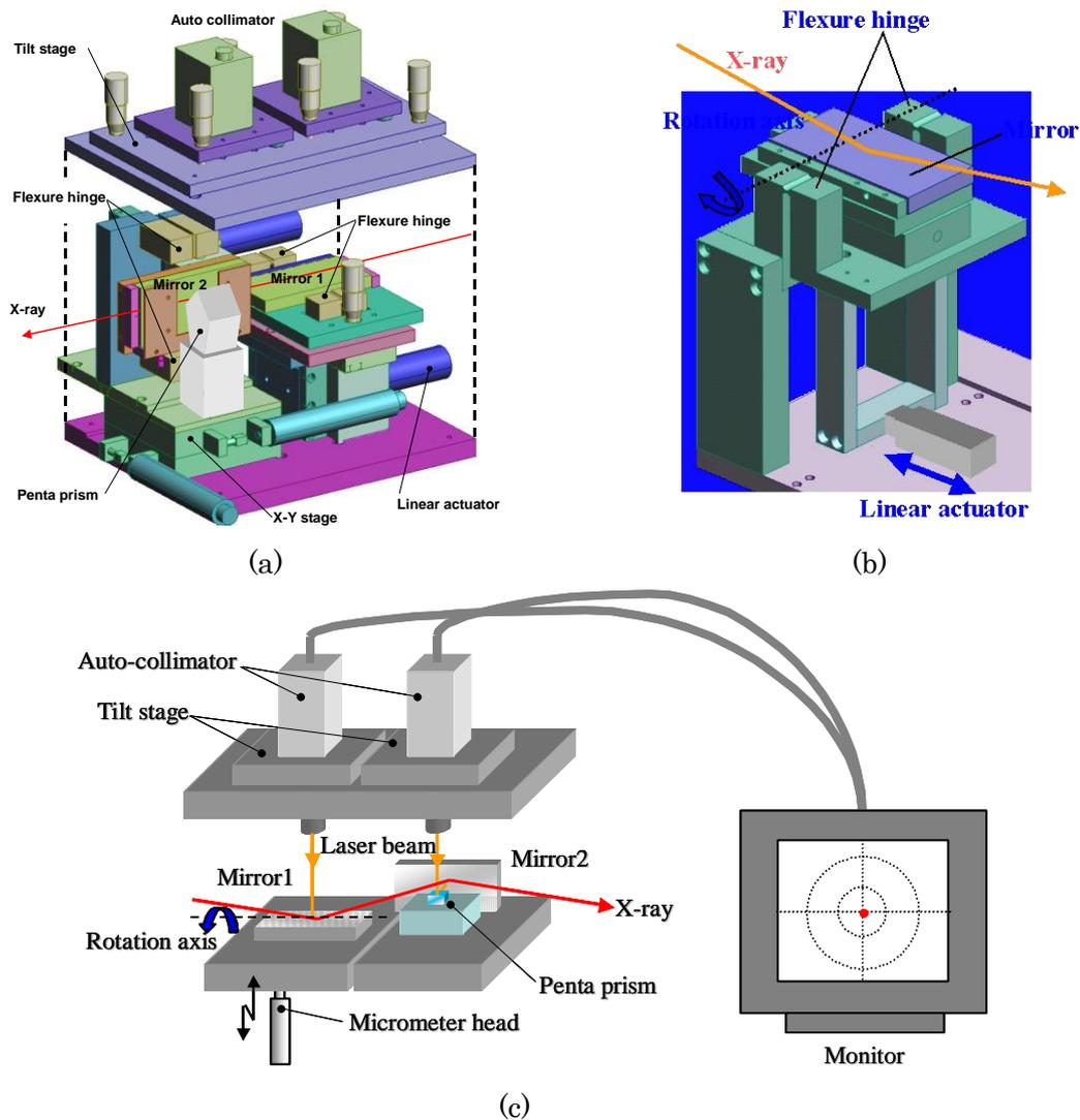
**Figure 5** (a) Mirror manipulator equipped with (b) glancing angle adjustment systems and (c) a perpendicularity adjustment system
