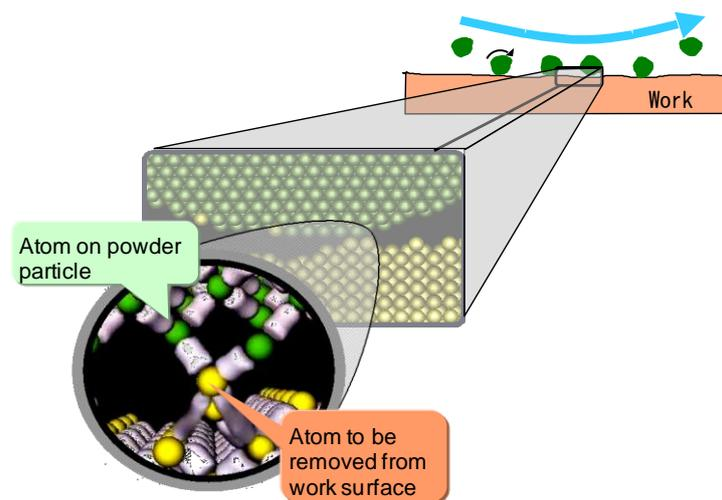
**Figure 2** Elastic emission machining (EEM). EEM is an ultraprecise machining method that utilizes the chemical reaction between the surfaces of the workpiece and fine powder particles. Topmost atoms on the workpiece will preferentially adhere to and move onto the surface of the powder particle. Eventually, atomically smooth surfaces can be obtained.
